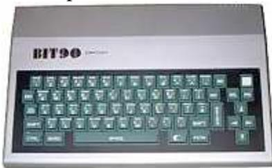
Developed in 1984, this computer was apparently never distributed via an official circuits in the west. Very largely inspired of the design and the hardware of Sega SC-3000. It is rumoured to be compatible with this system as well.
